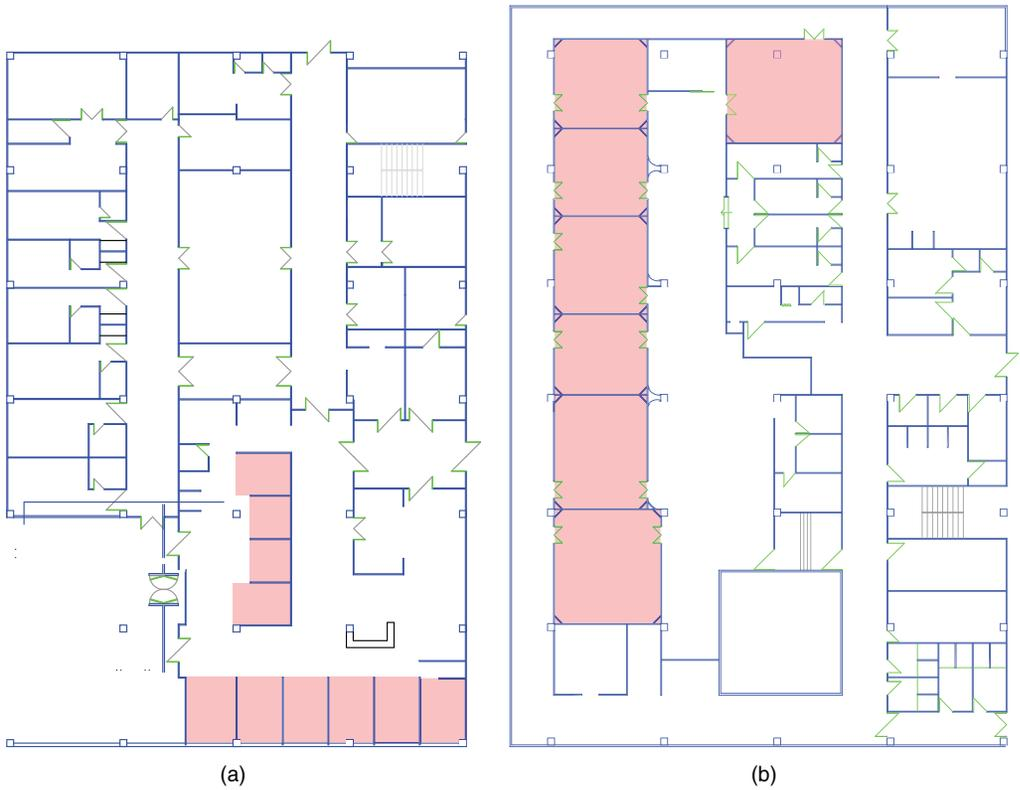
**Figure 4.** Two-story reinforced concrete frame building corresponding to the ED: (a) first floor with ten examination rooms, which contain a total of 13 examination stations; and (b) second floor with seven ORs, where the two least damaged are assigned to the ED.
